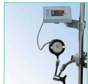
The centrifugal pump's compact size allows pole mounting of the entire system
