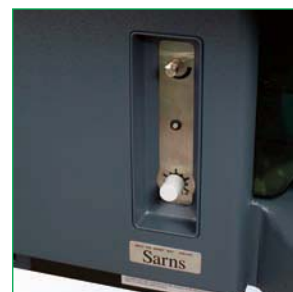
Electronic O 2 /air blender/analyzer housed in the base
