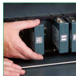
Modules plug into any of the available slots
